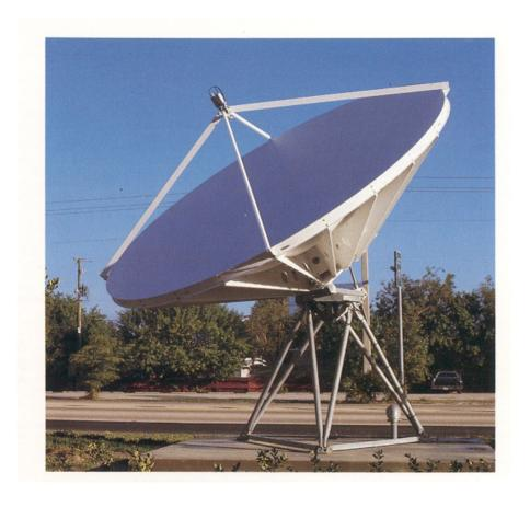
Prime Focus Feed; 5 meter reflector; Tx and Rx C-Band gain 46 dB; Beamwidth = 1° Ku-Band gain 54 dB; Beamwidth = 0.4°
