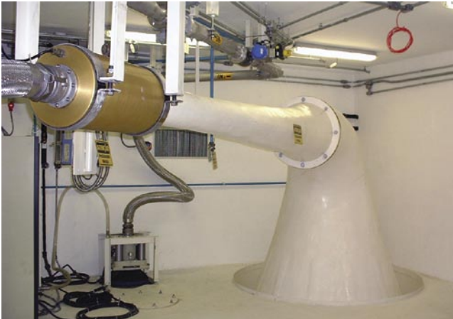
Figure 23-29 Generating through-the-ceiling high-intensity noise (courtesy of the Integration and Testing Laboratory, INPE, Brazil)
